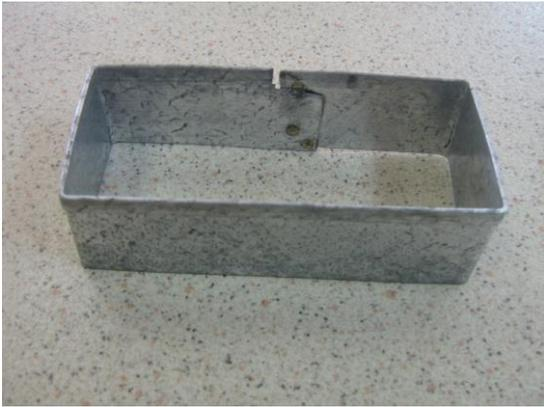
**Comment [Diocesan25]:** Metal frame constructed to make multiple bar and maintain consistent and uniform shape and size. This also helped us with time management and less manual labour and time effective than the vacuum formed mould
